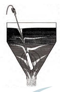
The paddle activator spreads the air vibrations deep into the material.
