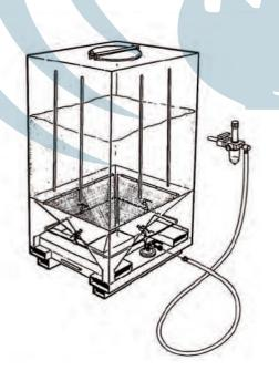
Sometimes, especially in smaller containers with difficult materials, it may be an advantage to have 3-4 very small Panel Activators operated by only one pulsator.
