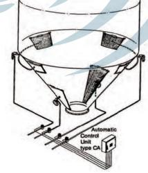
The activation should start automatically when the discharge begins. Otherwise there is a risk of discharging material in such a way that the activating surfaces are uncovered, forming a bridge above them. In larger silos, arcs are sometimes formed at the angle between
