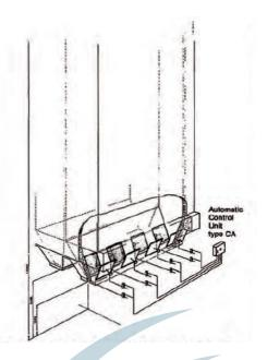
In this flour silo with a horizonally mounted discharging screw at the bottom, four pairs *of* Panel Activators above the outlet are activated in four stages, one after the other with 0.15sec. activating and 6-sec. idling period per working cycle, bringing the total air consumption down to only 50 litres/minute.
